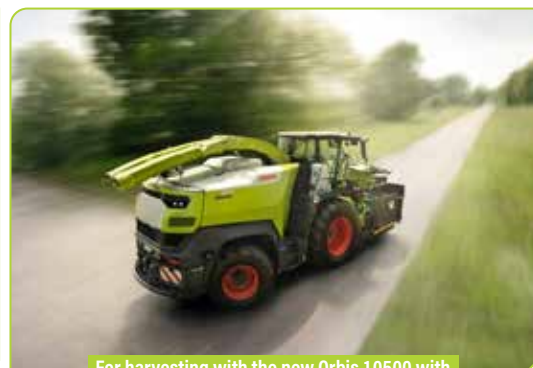
For harvesting with the new Orbis 10500 with maximum manifold length, the end piece can be folded hydraulically for safe road transport
