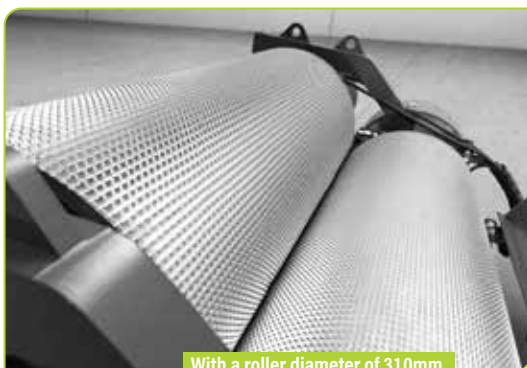
With a roller diameter of 310mm, the Multi Crop Cracker XL is the most powerful grain processor on the market.
