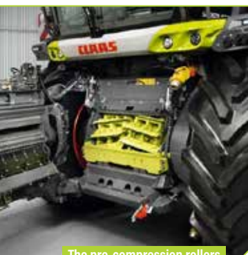
The pre-compression rollers ensure a uniform crop flow regardless of the layer thickness.
