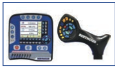
EC Tronic Control with Joystick or Optional VT Tronic Touch Screen Monitor ISOBUS ready
